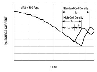
Figure 11. Reverse Recovery Time (t<sub>rr</sub>)
