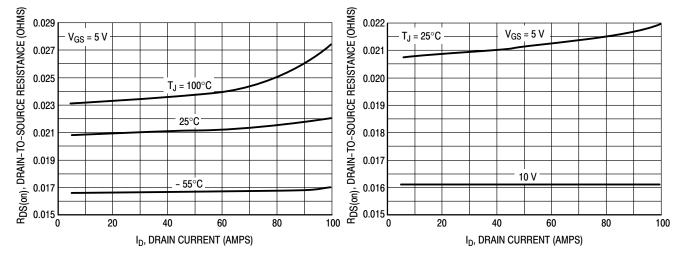
Figure 3. On-Resistance versus Drain Current and Temperature
