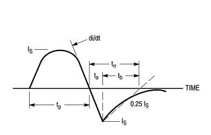
Figure 15. Diode Reverse Recovery Waveform
