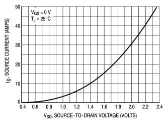
Figure 10. Diode Forward Voltage versus Current
