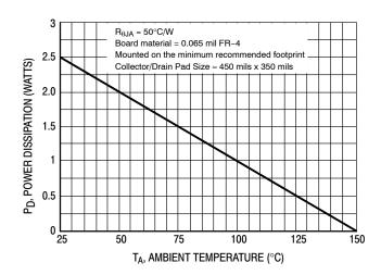
Figure 16. D<sup>2</sup>PAK Power Derating Curve
