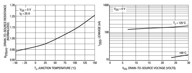
Figure 5. On–Resistance Variation with Temperature
